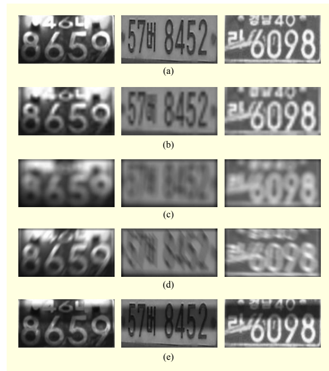
Fig. 2. Sample images in test database, including (a) original, (b) downsampled, (c) Gaussian blurred, (d) motion blurred, and (e) shadowed.
