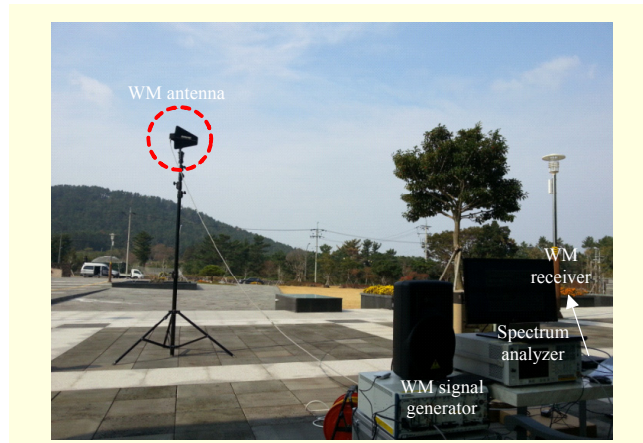
Fig. 6. Interference measurements from TVBD into WM receiver in front of Jeju Art Center in Korea.
