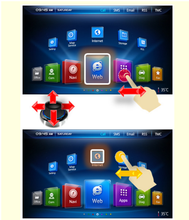
Fig. 4. UX based on four-directional movement: HMI UI manipulation is performed using knob or touch interface.
