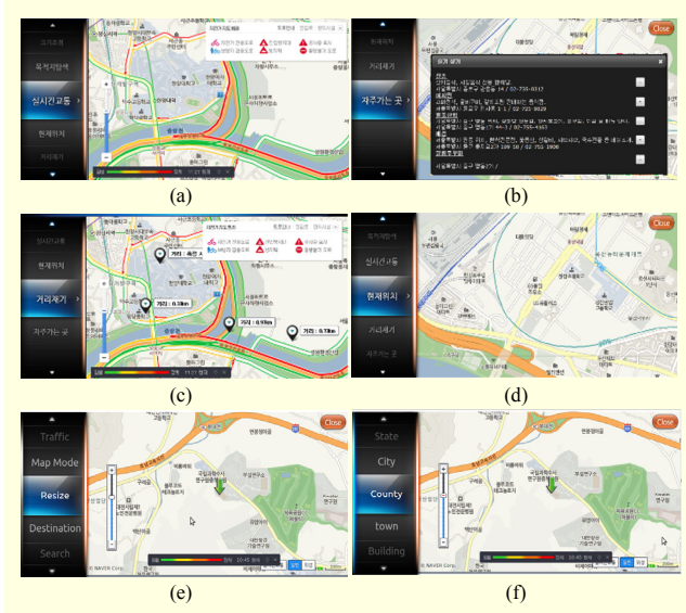
Fig. 9. Web-based map service based on UI framework: (a) real-time traffic status, (b) registered location, (c) measurement of distance, (d) setting current position, and (e) and (f) map resizing.
