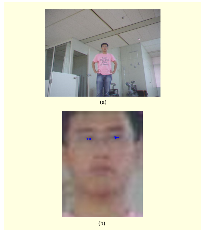
Fig. 8. (a) Original 320×240 image and (b) its face magnification. Note that making ground truth is difficult because most face components are significantly degraded. Also, center points of eyes are different between individuals.
