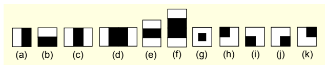
Fig. 2. Prototype simple features: (a)-(g) features proposed in [4] and [5] and (h)-(k) newly added features.
