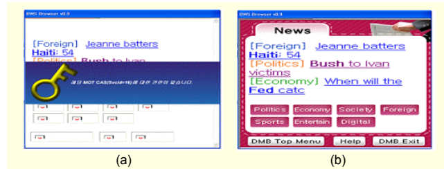
Fig. 7. Comparison of BWS service in MOT CA Mode: (a) without authorized key and (b) with authorized key.
