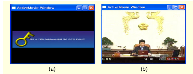
Fig. 6. Comparison of video service in subchannel CA mode: (a) without authorized key, and (b) with authorized key.
