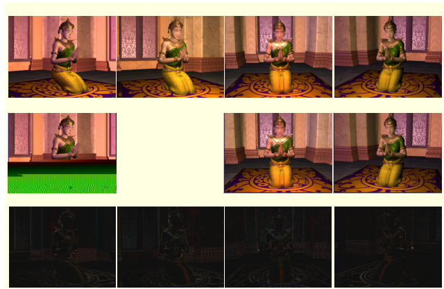
Fig. 10. Temple scene modeled with 1,404,052 polygons rendered from four different viewpoints: software-rendered images (top), relighted images (center), and difference images obtained by subtracting the center images from the top images (bottom). Nine cameras were used to cache the shading parameters of the scene.
