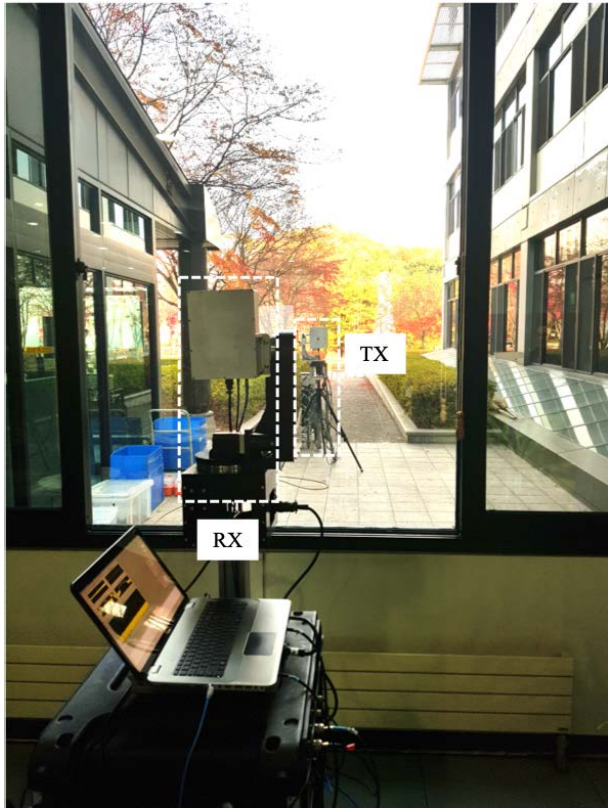
FIGURE 5. Glass window penetration loss measurement.
