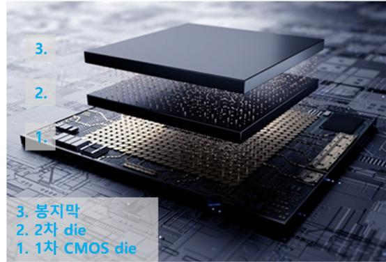
출처 Samsung Newsroom, “Samsung’s new 3D integration technology X-Cube(eXtended-Cube),” 2020, Reprinted with permission from Samsung.
