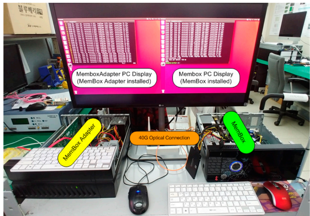
Figure 6. Access time measurement system.
