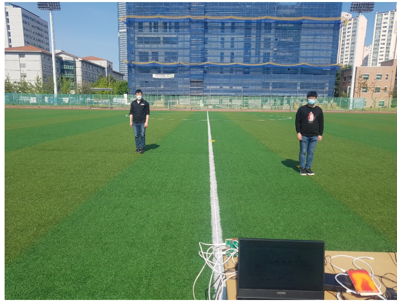
Figure 10. Experiment setup to measure the distributed FMCW radar signals.
