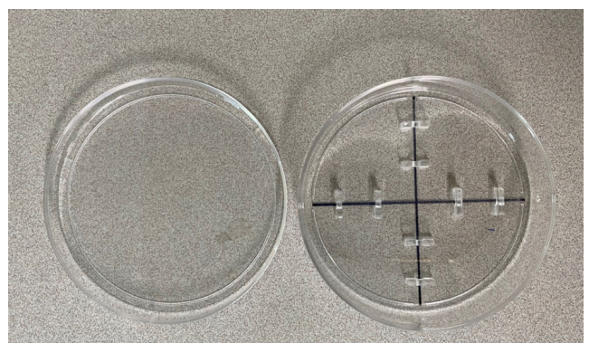
FIGURE 7. Testing jig for temperature measurements to ensure accurate thermometer placement.
