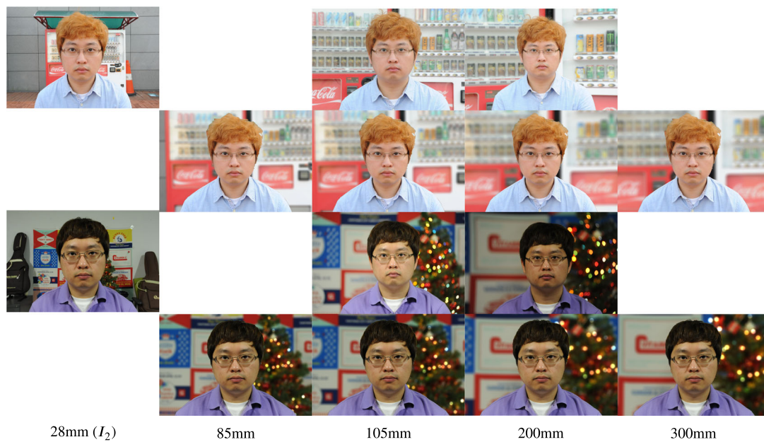
FIGURE 15 Examples of virtual view synthesis of the telephoto lenses, for the pairs of images. Top: images photographed using the specified lenses, bottom: images synthesized from the three rotating selfies
