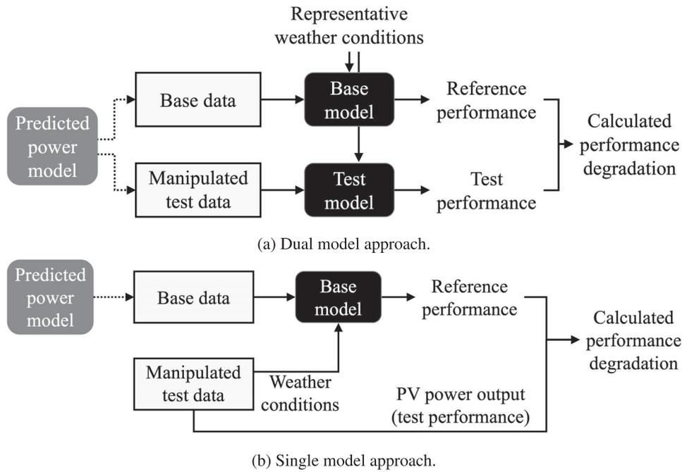
FIGURE 5 Two approaches of utilizing models to generate performance degradation
