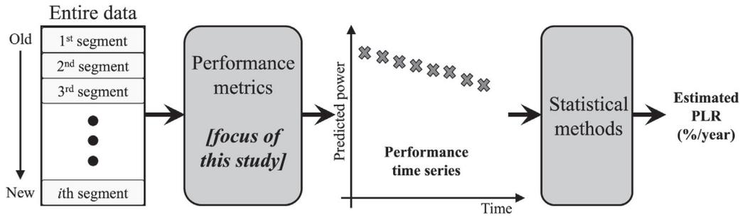
FIGURE 1 High-level illustration of PLR calculation
