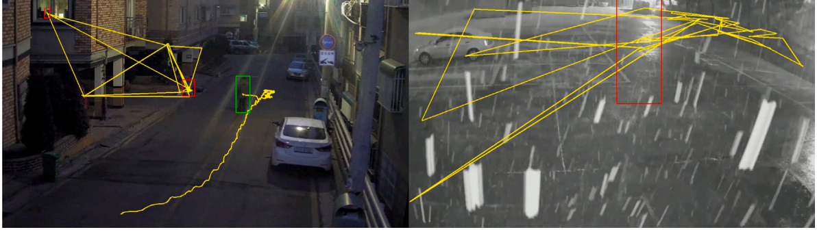
Fig. 3. Visualization of Human False Positive results. The bounding boxes and trajectories illustrate the observations from the human tracker, including instances where objects are misidentified as humans. These Human False Positives frequently occur in adverse environments such as low lighting as shown on the left and under severe snowstorm conditions on the right. The trajectories of incorrect instances demonstrate rapid and repetitive movements across long distances in random directions. Best viewed in color (Human: green bbox, False positive: red bbox, Trajectories: yellow lines).
