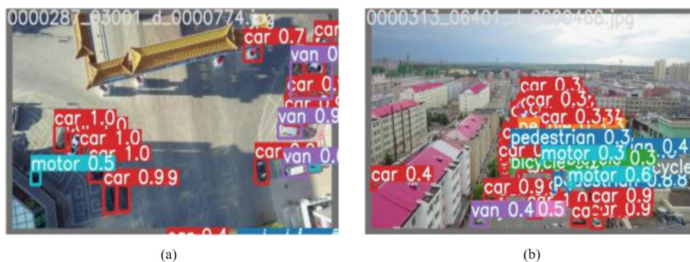
Fig. 4 Test results of DUA. The same model was used for testing. The model detect cars more accurately than motorcycles. However, the uncertainty for the car class can become higher with a few hard samples
