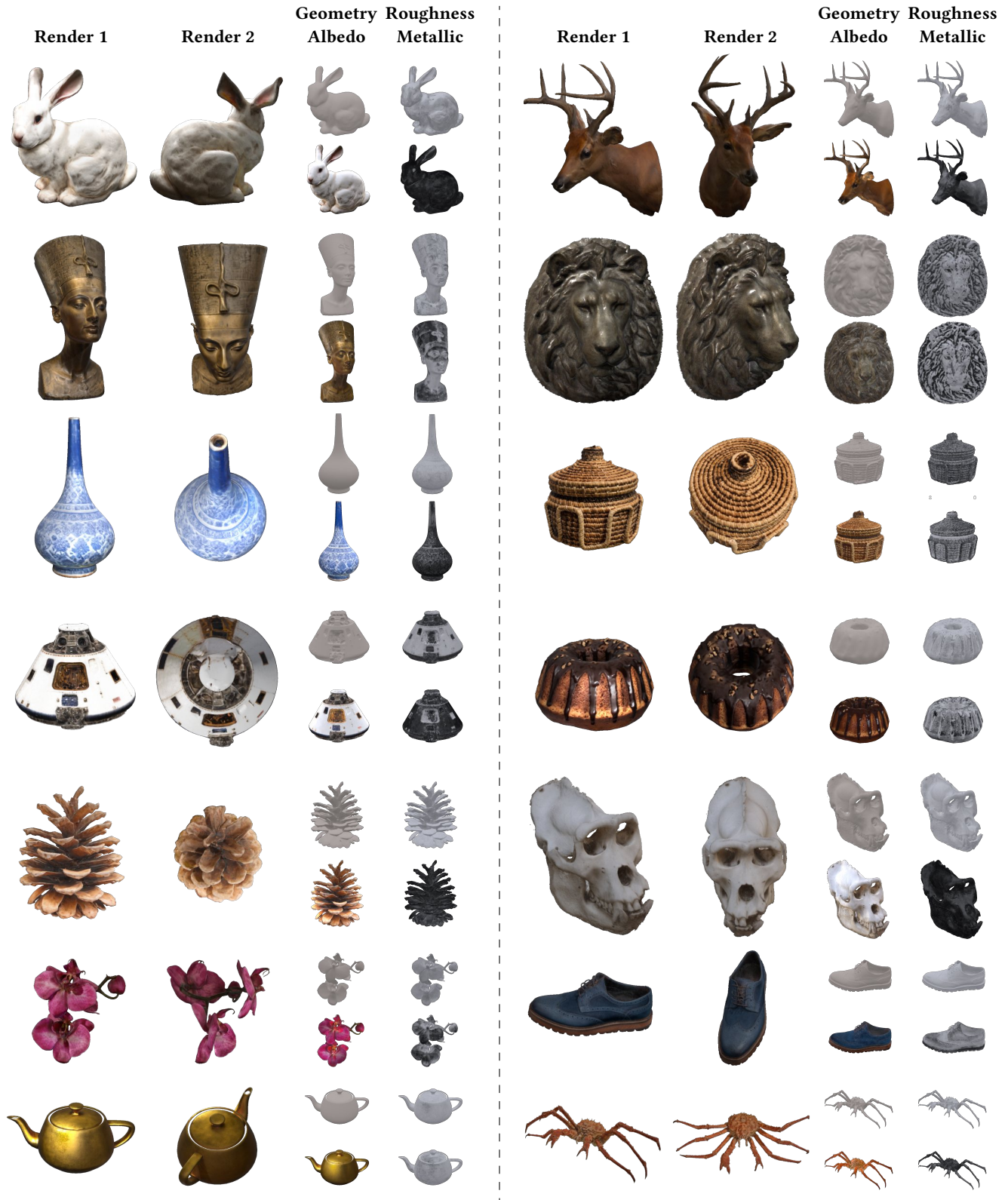
Fig. 10. Texture optimization results on diverse objects. For each example, we show two rendered views and the optimized PBR texture maps (albedo, roughness, metallic). Our method successfully handles a wide range of materials demonstrating strong generalization across object categories.
