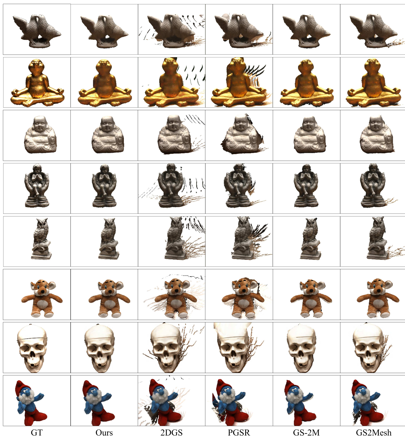
Figure 6. Qualitative mesh rendering results on the DTU dataset. Ground truth (GT), the proposed method (Ours), 2DGS, PGSR, GS-2M, and GS2Mesh are presented under corresponding viewpoints.
