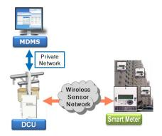
Figure 1. Architecture of the advanced metering infrastructure (AMI) system.
