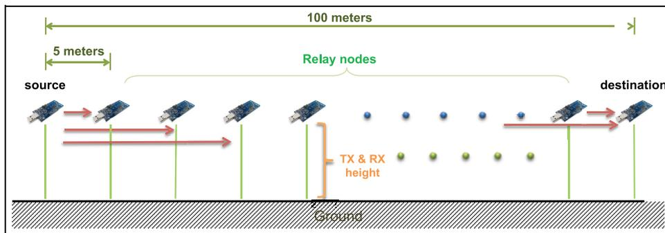
**Figure 4.** Multihop line topology experiment setup to measure the impact of deployment height on network depth and energy efficiency.
