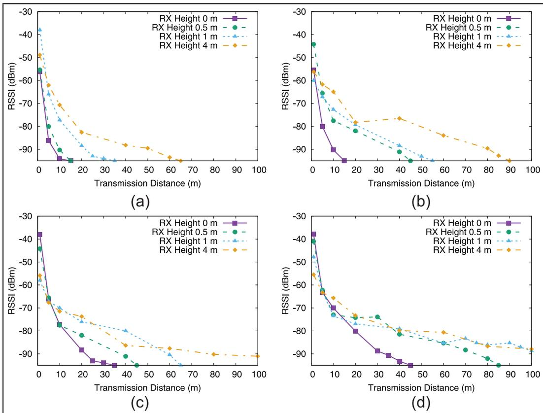
**Figure 2.** Received signal strength indicator (RSSI) value at the receiver versus transmission distance with varying heights of the transmitter and receiver: (a) TX height 0 m, (b) TX height 0.5 m, (c) TX height 1 m, and (d) TX height 1.5 m.
