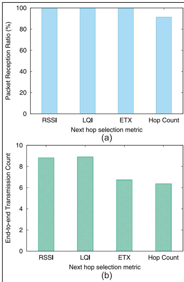
**Figure 8.** Performances from 20-node 100-m topology network installed at 0.5 m height with different link-quality measurement metrics: (a) packet reception ratio (PRR) and (b) total number of packet transmissions.
