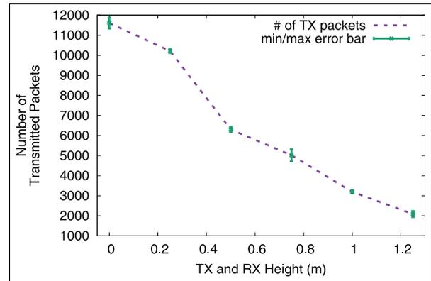
**Figure 5.** Total transmission packet count for sending 1000 end-to-end packets on a 100-m line topology of 20 nodes with varying installation heights from 0 (ground) to 1.25 m at 0.25 m interval (same height for both transmitter and receiver).
