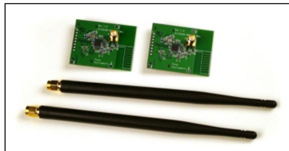
**Figure 6.** CC1200 radio module used in our experiments.
