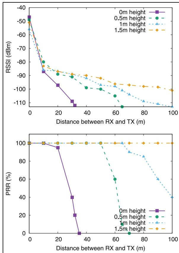
**Figure 7.** RSSI and PRR performance of CC1200 radio at 900 MHz versus transmission distances with varying heights for both the transmitter and receiver.
