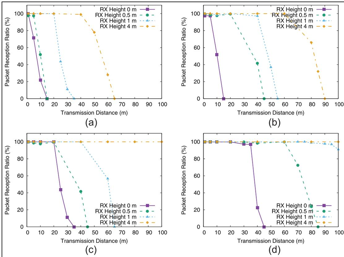
**Figure 3.** Packet reception ratio (PRR) at the receiver versus transmission distance with varying heights of the transmitter and receiver: (a) TX height 0 m, (b) TX height 0.5 m, (c) TX height 1 m, and (d) TX height 1.5 m.
