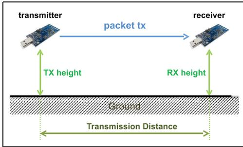
**Figure 1.** Single-hop experiment setup to measure the impact of deployment height on transmission range and connectivity.
