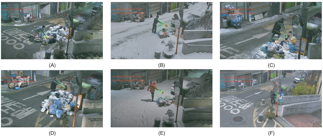
FIGURE 8 Qualitative results of dumping action. The red messages at the top left indicate that the proposed method detected a dumping action
