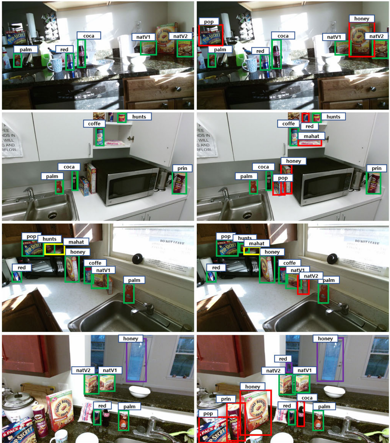
FIGURE 6. Detection results of the original cut-and-paste method (left) and our final method (right). The detection model trained on our generated dataset is more robust to variations in the object instances, such as occlusions and illuminations, with tight bounding-boxes (See red and yellow boxes). However, our method is more vulnerable to false acceptance error (purple boxes).
