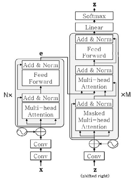
Fig. 1. Block diagram of the Transformer-based ASR model.
