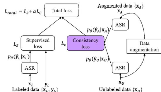
Fig. 2. (Color available online) Training objective for UDA, where ASR is a trained baseline model that predicts a distribution of  $\hat{\mathbf{y}}_A$  given  $\mathbf{x}_A$  and  $\hat{\mathbf{y}}_U$  given  $\mathbf{x}_U$ .
